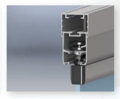
**Top Telescopic Profile**The top telescopic profile absorbs any building irregularities in height up to 25mm. It is easy to install and regulate.
